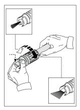
17. Spray pattern shape and intensity can be changed by twisting the spray adjuster at the end of the lance. KEEP HANDS CLEAR OF THE FRONT OF THE LANCE TO PREVENT INJURY. NOTE: Turbo nozzle is not adjustable.
