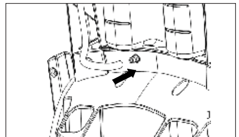
Figure 10 - Attach soap tube to unit (models PW1825 and PW1835 only)
