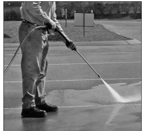
Figure 22 - Optimum angle to cleaning surface
