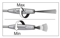
➔ To apply detergent, the wand must be positioned to the lower pressure setting (Mix).
