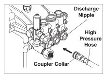
**STEP 8:** Connect the high pressure hose to the discharge nipple. Push coupler collar forward until secure.
