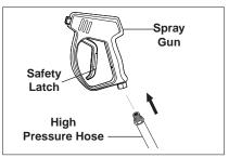
**STEP 4:** Attach the high pressure hose to the spray gun using teflon tape on hose threads.
