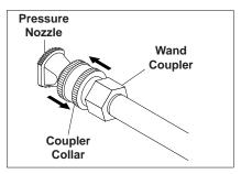
**STEP 7:** Release the coupler collar and push the nozzle until the collar clicks. Pull the nozzle to make sure it is seated properly.
