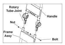
**STEP 1:** Insert rotary joints into frame tubes so that stops point away from engine. Then fix them using 1/4" bolts and nuts on each side and tighten.
