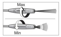
→ To apply detergent, the wand must be positioned to the lower pressure setting (Mix).
