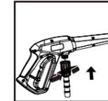
2b) Connect the high pressure hose to the trigger handle. Refer to manual for further details.
