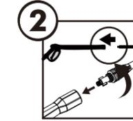
2a) Assemble pressure washer gun top half to bottom half
