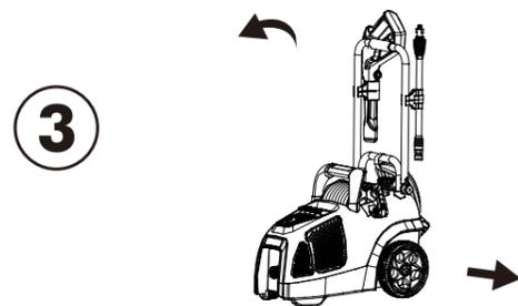
• Close for storage: Pull out on the locking pin at base of handle. Fold handle bar forward to front of unit.
