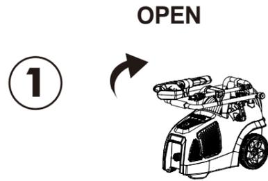
• Open for use: Lift up on the handle bar pivoting it towards the back into an upright position until it clicks and locks into place.
