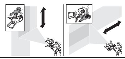
Trigger gun after starting the stroke. Release the trigger before ending the stroke.
