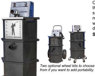
Capture and transfer up to 3000 gallons of water per hour with the RPV Hydro Vacuum® water & flood recovery vacuum systems. They feature a powerful, industrial 2-stage vacuum motor and a heavy duty stainless steel water pump to transfer wastewater while vacuuming continues... no need to stop and dump the collection tank. Dimensions: 17"W x 38"H, 56 pounds
