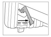
After engine has warmed and idles smoothly, move CHOKE lever to the RUN position as indicated.
