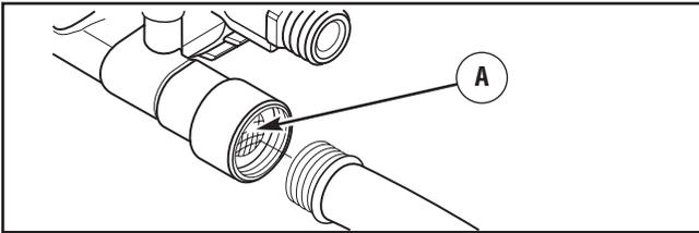
5. Connect the garden hose (not to exceed 50 feet (15 m) in length) to the water inlet. Tighten by hand.
