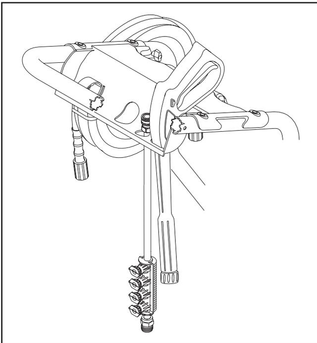
2. Place spray gun through hole on accessory tray on right side of unit.
