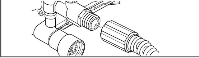
3. Run water through your garden hose for 30 seconds to clean out any debris.
