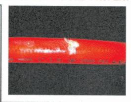
LIKE STRANDS IN A BRIDGE CABLE, EACH REINFORCEMENT FIBER PLAYS AND EXACT ROLE IN THE ULTIMATE BURST STRENGTH OF THE HOSE. A MINOR SLICE OR NICK IN THE REINFORCEMENT CAN RESULT IN TOTAL HOSE FAILURE.
