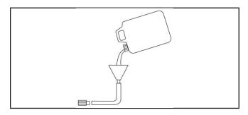
Pour the antifreeze into the funnel, then pull on the engine recoil starter to create suction in the pump housing. Pull the recoil several times until antifreeze comes out of the pump outlet.
