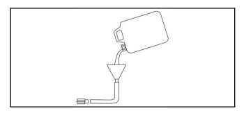
5. Pour the antifreeze into the funnel, then pull on the engine recoil starter to create suction in the pump housing. Pull the recoil several times until antifreeze comes out of the pump outlet.
