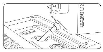
6. Screw on the fuel cap and wipe away any spilled fuel.
