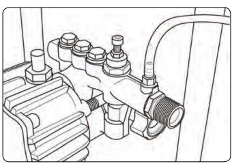
Place the filter end of the detergent hose into pressure washer detergent (not included).
