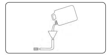
5. Pour the antifreeze into the funnel, then pull on the engine recoil starter to create suction in the pump housing. Pull the recoil several times until antifreeze comes out of the pump outlet.
