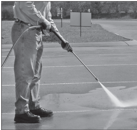
Figure 12 - Optimum angle to cleaning surface
