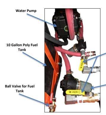
**Ball Valves for Water Supply Lines to Pump**
