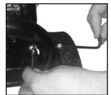
6. Assemble the upper gun hook using (1) M6 x 45mm long socket head cap screw, (1) M6 nut, and the supplied hex wrench and openend wrench. Tighten securely.
