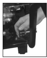
5. Assemble the lower gun hook using (1) M6 x 45mm long socket head cap screw, (1) M6 nut, and the supplied hex wrench and openend wrench. Tighten securely.
