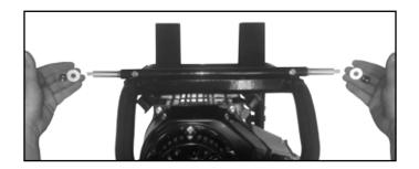
Remove (1) M8 washer and (1) M8 nut from wheel axle and place wheel onto axle.
