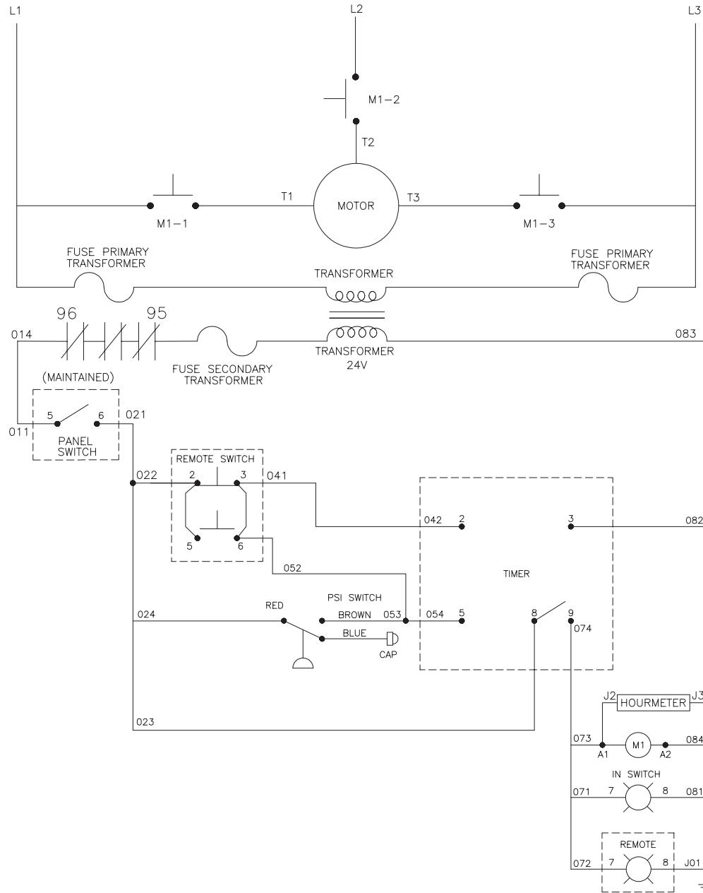
WIRING DIAGRAM THREE PHASE - REMOTE BOX (AFTER SERIAL #11346043)
