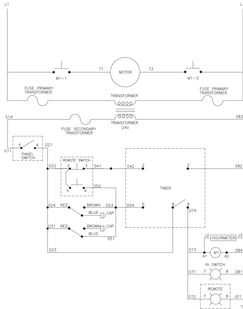
WIRING DIAGRAM SINGLE PHASE - AUTO START/STOP, REMOTE BOX (AFTER SERIAL #11351284)
