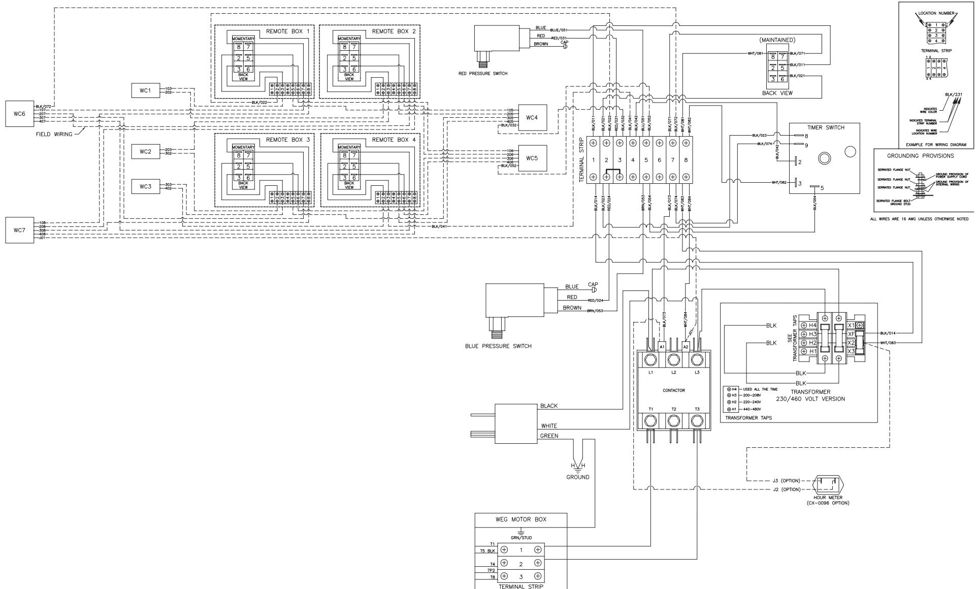
WIRING SCHEMATIC THREE PHASE - AUTO START/STOP, MULTI REMOTE BOX (AFTER SERIAL #11346043)
