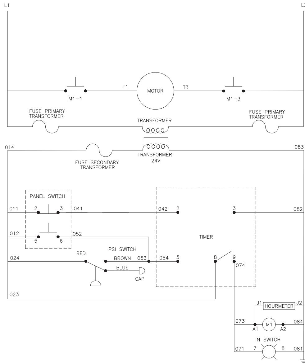
WIRING DIAGRAM SINGLE PHASE (AFTER SERIAL #11351284)
