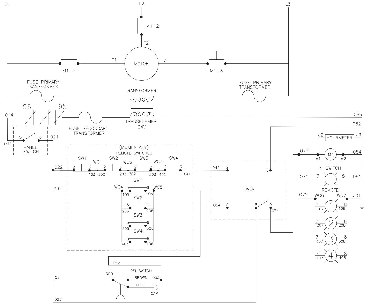
WIRING DIAGRAM THREE PHASE - MULTI REMOTE BOX (AFTER SERIAL #11346043)
