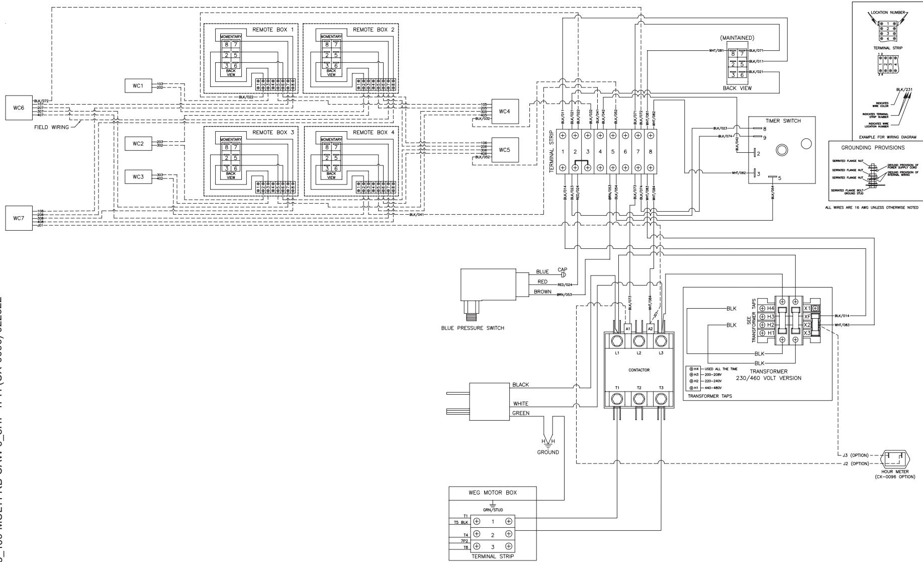
WIRING SCHEMATIC THREE PHASE - MULTI REMOTE BOX (AFTER SERIAL #11346043)
