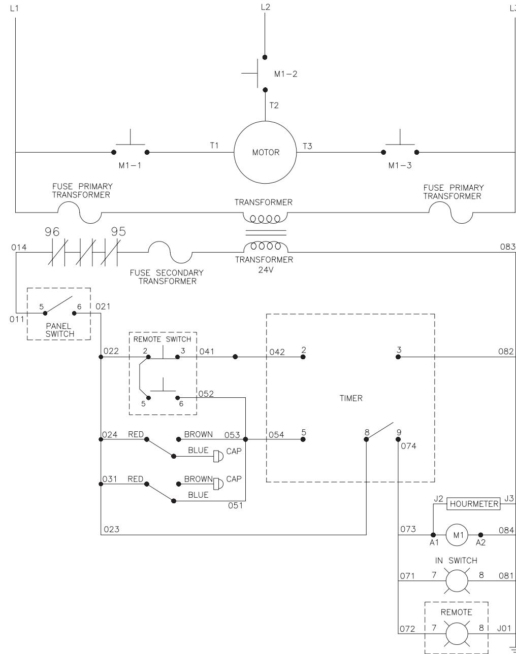
WIRING DIAGRAM THREE PHASE - AUTO START/STOP, REMOTE BOX (AFTER SERIAL #11346043)
