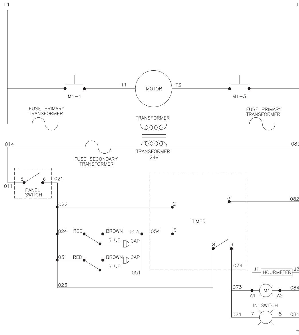
WIRING DIAGRAM SINGLE PHASE - AUTO - START/STOP (AFTER SERIAL #11351284)
