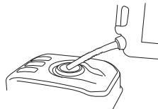
Figure 2-7. Add Recommended Fuel
