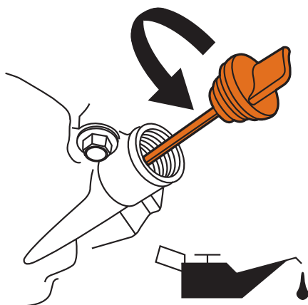
Figure 30 – Fill Engine Oil
