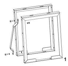
1) It's easiest if the BRACE is bolted to the ASSEMBLY FRAME first. If you have a DHRA50300 use the brace p/n 2540095; if you have a DHRA50150 use the brace p/n 2540096, if you have a DHRA50450 use the brace p/n 2540105. Do not tighten these bolts yet. Use (2) M8 nuts and bolts and (4) M8 washers. Be sure the cutout in the frame is on the bottom.
