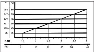
Naturally, if the application allows for feeding the pump with 45 psi (3 bar) even at low temperatures (for example: 115<sup>O</sup>F/45<sup>O</sup>C the life of the wet end of the pump will be even longer.
