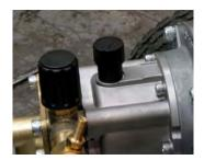
Install black oil plug in top of pump before attempting to start and run pump.
