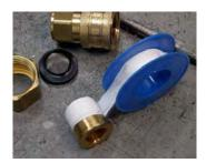
Apply Teflon tape to threads of inlet nipple
