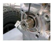
Using a 5/32" allen wrench, remove the set screw holding drive gear onto engine crankshaft.
