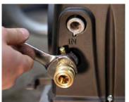
Remove filter from inlet nut, and using a 3/8" allen wrench or socket, unscrew the inlet fitting from the pump.
