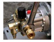
Screw quick connect fitting onto chemical injector.
