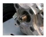
Place key in groove on engine shaft.
