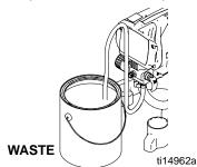
7. Submerge suction tube in water or flushing solvent.
