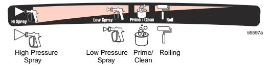
NOTE: To select function, align symbol on pressure control knob with setting indicator on sprayer.
