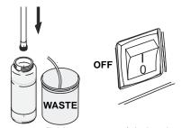
When storage fluid comes out of drain tube, turn power switch OFF.
