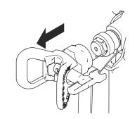
With the trigger safety ON, remove tip and guard from gun and place into waste pail for further cleaning.
