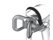
Install tip and guard on gun, and hand tighten. Your are now ready to spray.
