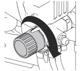
Turn Pressure Control Knob right (clockwise) to increase pressure at the gun, and turn it left (counterclockwise) to decrease the pressure.
