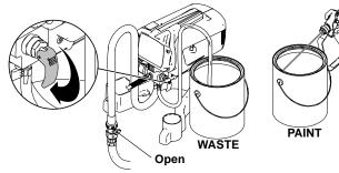
Trigger gun into paint pail and lower spray/prime valve to SPRAY. Turn power switch ON to push paint in hose into paint pail. When water comes out of the gun, keep gun triggered and move aim of gun into waste pail.
