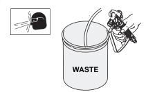
When paint comes out of gun, release trigger. Pump will build up pressure, and motor will stop.
