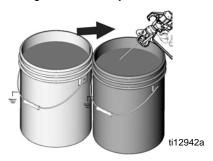
14. Stop triggering gun. Engage the trigger lock.
