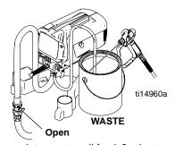
Trigger gun into waste pail for 1-2 minutes until relatively clear water comes out of gun.
