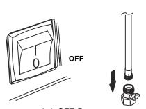
Turn power switch OFF. Remove power flush attachment from suction tube.
