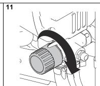
Turn pressure control knob to right (clockwise) until pump starts.
