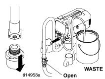
Unscrew inlet screen from suction tube. Thread power flush attachment onto suction tube.
