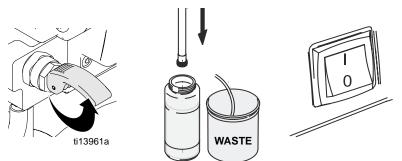
Submerge suction tube and drain tube in storage fluid. Always use Graco pump armor or mineral spirits/paint thinner for storage fluid. Lift spray/prime valve to PRIME. Turn power switch ON.
