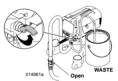
Lift prime/spray valve to PRIME. Let water flow through the sprayer and into waste pail for 20 seconds.
