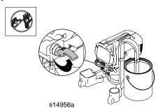
Turn power switch OFF. Place suction tube and drain tube into empty waste pail. Lift spray/prime valve to PRIME to relieve fluid pressure.
