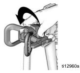
2. Uncoil hose and connect one end to gun. Use two wrenches to tighten securely.
