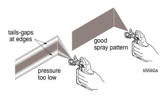
**NOTE:** If tails persist when spraying at the highest pressure, a smaller tip is needed or the material may need to be thinned.
