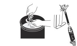
Clean tip, guard and inlet screen with a brush. Remove filter from spray gun, and clean with a brush. Reassemble spray gun guard/tip and filter.
