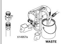
Thread power flush attachment onto garden hose. Rinse paint off of suction tube, drain tube and inlet screen.
