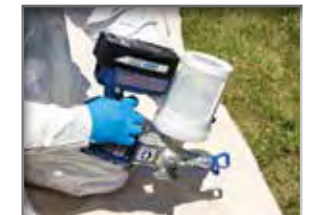
Attach cup with solvent, set to "Clean" and run upside down.
