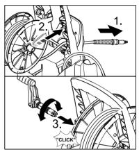
Install the holder bracket and secure it using 2 screws.
