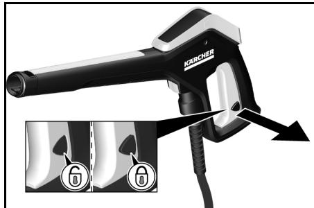
3. Set the high-pressure gun with the spray lance in the parking position.
