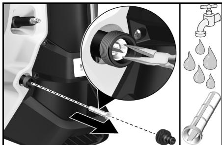
4. Insert the sieve into the water connection.
