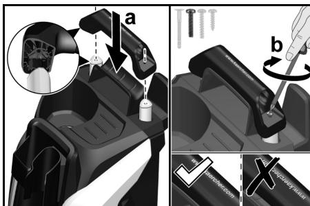
2. Secure the transport handle with 2 screws.
