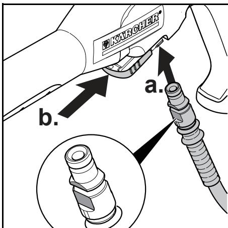
3. Push the locking slide into the trigger gun until fixed into place.
