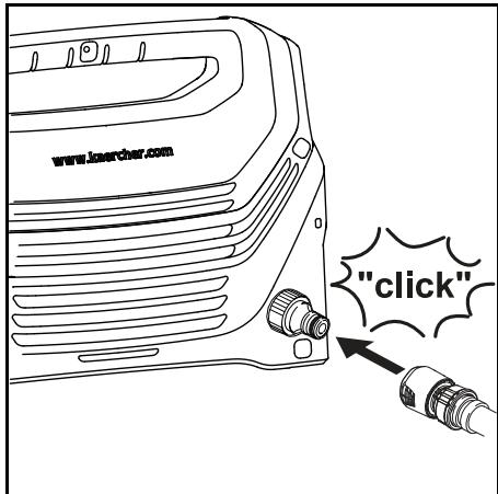
3. Connect the water supply hose to the water supply.
