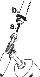
3. Connect the foam cannon to the trigger gun, and turn the foam cannon by 90° to lock it.
