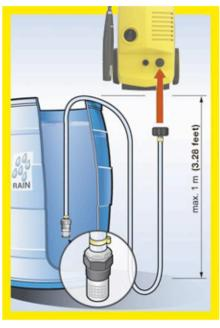
The water suction hose is 3m (9.8 feet) in length and can draw water from a standing source up to 1m (3.28 feet) below the pressure washer. These modifications are for U.S./Canadian residential pressure washers only. \*Adapter (A) is available at BuyKarcher.com. Hose clamp can be purchased at most hardware stores.
