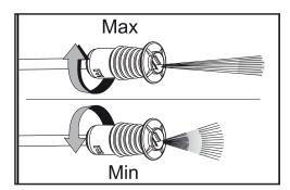
→ For lower pressure turn the wand collar in the minus (Min) direction.
