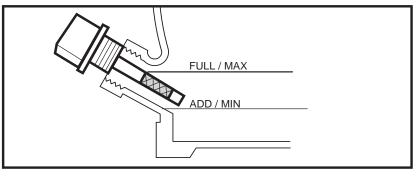
Be sure the machine is level when checking the oil level. (Refer to the engines operating manual for seasonal grades).
