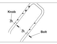
**STEP 2:** Insert the carriage bolt through the holes from the back of the unit and attach a knob from the front of the machine. Tighten Knobs with by hand.
