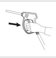
**STEP 5:** Trigger the spray gun to eliminate trapped air then wait for a steady flow of water to emerge from the spray nozzle.
