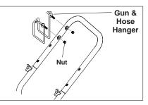
**STEP 3:** Attach the Gun & hose hanger and insert nuts from inside. Tighten nuts.
