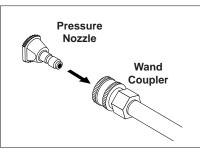
**STEP 7:** Pull spring-loaded collar of the wand coupler back to insert your choice of pressure nozzle.
