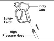
**STEP 5:** Attach the high pressure hose to the spray gun using teflon tape on hose threads.
