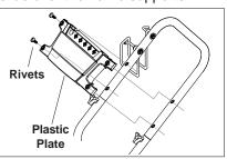
**STEP 4:** Attach the plastic plate from the top aligned to the four holes placed on top of the handle and insert the rivets through holes of plastic plate.
