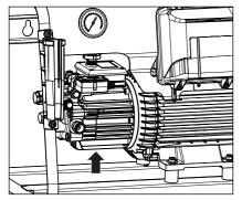
The first oil change should be carried out after approximately **50 operating hours**, then every year or after 250 operating hours. If the oil turns grey or white, you must change the oil. In case of exchanging oil being required, the oil drain screw must be opened above a container and the high pressure cleaner be emptied. The oil is to be caught in the reservoir and disposed of in an approved manner.
