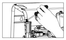
Fasten the holders for the lances using a Phillips head screwdriver and the screws enclosed.
