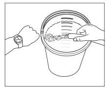
Lack of water occurs more often than you probably believe. The more powerful a high pressure cleaner is the greater is the danger that a lack of water occurs. If there is only an insufficient amount of water available, cavitation (water-gas mixture) arises inside the high pressure pump, which is normally noticed too late or even not at all. **The high pressure pump will be destroyed.** Please check the available quantity of water by filling a bucket with liter scale for one minute.
