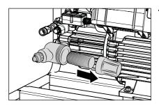
If using a water inlet filter check it for cleanliness prior to each startup.
