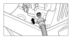
**1.** Mount suction hose with suction filter (Kränzle accessories No. 15.038 3). When using other hoses the inner cross section of the hose must be at least 3/4" = 16 mm.
