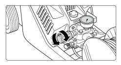
**11.** Connect to circuit. **Kränzle 2017, 2017 T: 115 V ~, 60 Hz Kränzle 2020, 2020 T: 115 V ~, 60 Hz** The socket must be protected For K2017, K2017T with a 15A or 16A delay action fuse on the mains side. For K2017, K2017 T, K2020, K2020 T with a 20A delay action fuse on the mains side.
