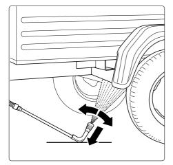
Always aim the underbody lance! Bear in mind when using a curved or angled spraying lance that there is a significant amount of torque in the recoil!
