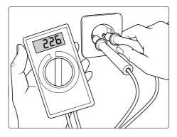
If there are too many collectors in your proximity connected to the network at the same time, the available voltage and the current intensity may decline. Consequently the motor of the high-pressure cleaner does not start or even blows.
