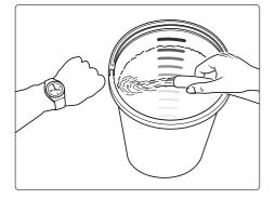
Lack of water occurs more often than you probably believe. The more powerful a high-cleaner is the greater is the danger that a lack of water occurs. If there is only an insufficient amount of water available, cavitation arises inside the pump, which is normally noticed too late or even not at all. **The pump will be destroyed!** Please check the available quantity of water by filling a bucket with litre scale for one minute.
