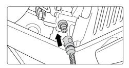
**10.** Connect water hose to water tank. The cleaner may be connected to water mains with cold or 60°C warm water. Alternatively water can be sucked in from a container (see page 17).
