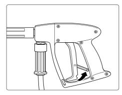
Apply the safety catch on the trigger gun after each use, in order to prevent unintentional spraying!
