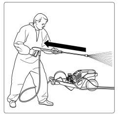
Bear in mind that during cleaning tasks with a high-pressure water jet a significant recoil at the lance arises (see technical data on page 4).
