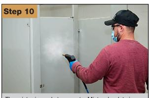
The mister is ready to operate. Mister droplet size -20-30-micron at 2-inches from tip at 350-PSI.
