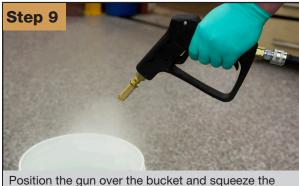
Position the gun over the bucket and squeeze the trigger. Detergent should be dispensing through
