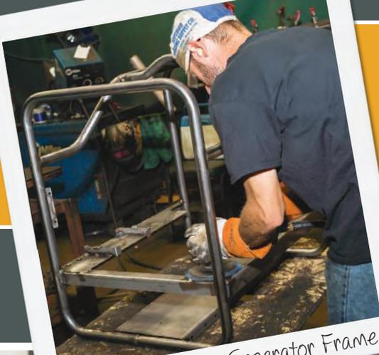
Finishing Work on Generator Frame
