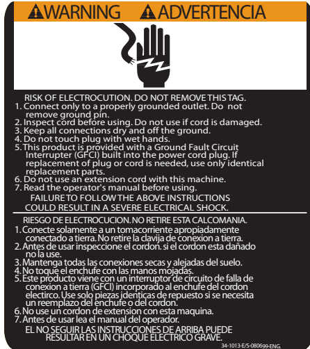
Reference #20A Decal: Warning-Risk of Electrocutation (Part # 34-1013)
