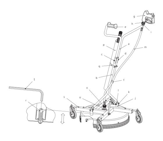
Slide the upper fork (a) over the lower fork (b). Secure the two forks with the bolt (c) and the safety nut (d).
