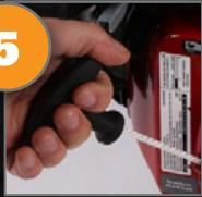
Pull recoil lightly until resistance is felt then pull in one fast motion.
