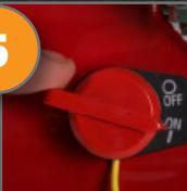
Place the On/Off switch to the "On" position and place the fuel tab to the "On" position
