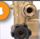
Connect high pressure hose to quick connect inlet and attach wand to the gun.
