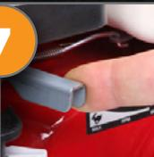
Move the throttle lever to the slow position, about 1/3 of the way toward the fast position.
