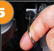
Set choke to the closed position for a cold start.
