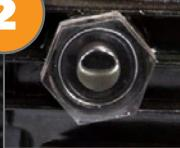
Fill pump with SAE 30 (non detergent) oil until filled half way through the sight glass.
