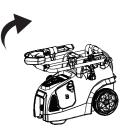
• Open for use: Lift up on the handle bar pivoting it towards the back into an upright position until it clicks and locks into place.
