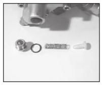
2. Remove the valve spring (18) and valve cone (36) from the manifold (35). Inspect the parts for wear and replace as necessary.
