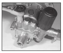
1. With a 14mm socket wrench, remove the three discharge valve plugs (22). Inspect the valve plug o-rings (23) for wear, and replace as necessary.
