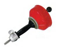
pplicable for both indoor and outdoor small drain pipes (1-1/4" to 3"), Shark's drain augers are designed to be simple to use and easy to handle. Simply release the locking screw, insert the soft Ashaft into the pipe, latch the lock and rotate the handle. The metal barrel core ensures cleaner and more convenient use.
