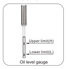
4. Completely insert the dipstick into the dipstick hole during inspection.
