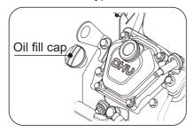
3.Remove the dipstick and check the oil filling volume which should be at the upper limit of the scale (H point).
