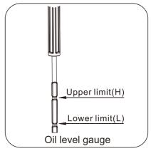
Fill to the upper limit (marked with "H") of the dipstick with the recommended oil if the oil level is low.
