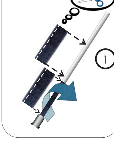
**Step 1:** Remove film from back of 2" x 5" loop piece and place around pressure washer wand just above the spray nozzle. On 1/2" wands trim 1/4" width so no overlap is produced. Once loop piece is attached to the wand, **allow 12 hours for adhesive to cure for most secure bond**. A second loop piece is also provided and may be used if necessary for more adjustability and closer proximity of spray to surface.
