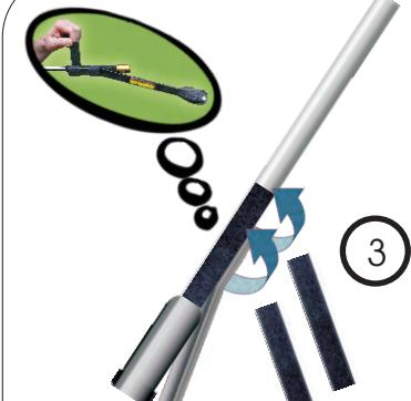
**Step 3:** Attach 1"x 6" hook and loop straps around both the wand and Sprayglide™. We recommended you start this wrapping procedure by attaching the strap to the loop material adhered to the wand in step 1. This will provide stronger grip when you pull to secure tightly around the wand and Sprayglide™ together.
