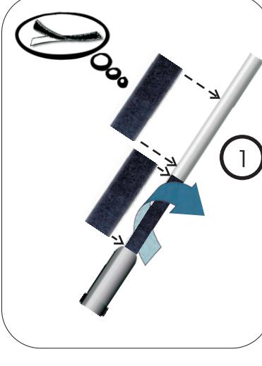
**Step 1:** Remove film from back of 2"x 5" loop piece and place around pressure washer wand just above the spray nozzle. Once loop piece is attached to the wand, **allow 12 hours for adhesive to cure for most secure bond**. A second loop piece is also provided and may be used if necessary for more adjustability and closer proximity of spray to surface.
