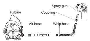
IMPORTANT: Do not attach the short air whip hose directly to the turbine, as the hose will become damaged.
