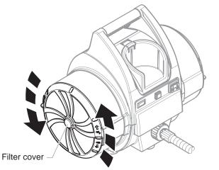
2. Remove each filter set (pre-filter and filter) from the filter housing on each side of the turbine.
