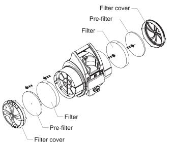
3. Clean the filters. Either tap the filters to knock out the contaminants or use pressurized air to blow out the contaminants. For material that is not blown or knocked loose easily, soak the filters in soapy water or mineral spirits. Allow the filters to dry completely before placing them back in the turbine.
