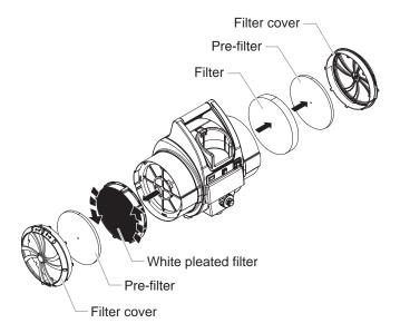
Clean the filters. Either tap the filters to knock out the contaminants or use pressurized air to blow out the contaminants. For material that is not blown or knocked loose easily, soak the filters in soapy water or mineral spirits. Allow the filters to dry completely before placing them back in the turbine.
