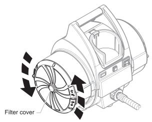
Remove each filter set (pre-filter and filter) from the filter housing on each side of the turbine.
