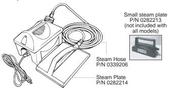
NOTE: The water container, heating element and hose are not serviceable. Should a problem occur with the steamer, contact Wagner Technical Service.
