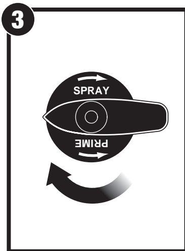
3. Make sure the PRIME/SPRAY knob is turned to SPRAY. Unlock the spray gun.
