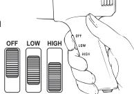
IMPORTANT: If the blower motor in the heat gun does not turn on when the switch is set to either LOW or HIGH, turn the switch OFF immediately. The heating element will burn out if it is not cooled by the blower.
